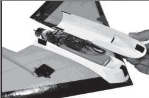
Cut two of the 1" X 1" Velcro pieces in half. Apply the loop side of the Velcro to the front and rear sides of the motor tray. Apply the hook side to the inside of the canopy opposite the loop side.
