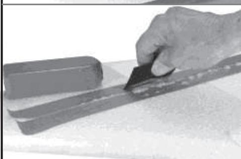
Use a piece of plastic as a squeegee to work the glue into the spar slot. Spray both sides of the spar with glue and press it into the channel while the glue is wet. Use the squeegee to press the spar to the bottom of the channel. Squeegee any overflow glue back into the channel over the buried spar. Let the glue set for at least 4 hours with the weights in place. Overnight is even better
