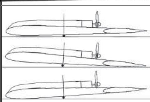
Place the wing right-side-up on a flat surface. Balance is achieved when the wing stays in the nose up and nose down positions. Nose weight is usually not necessary but an ounce or so may be used if necessary. See The website [zagi.com](http://zagi.com) for video building tips.
