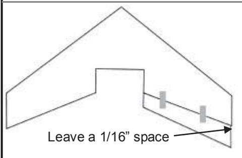
Place the wing in the bottom beds, top side up. Place weights on the wing. Position the elevator against the trailing edge of the wing. The wide end of the elevator goes out-board. Align a straightedge with the wing tip. Leave a 1/16" space between the end of the elevator and the wing tip. Make a placement reference mark on the TE of the wing at both ends of the elevators.
