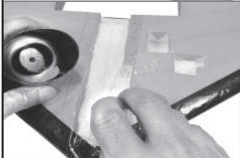
Make a glue slurry in a cup. Apply glue inside the pencil line. Brush the glue onto the motor tray cutout floor. Do not apply adhesive to the vertical walls of the cutout.
