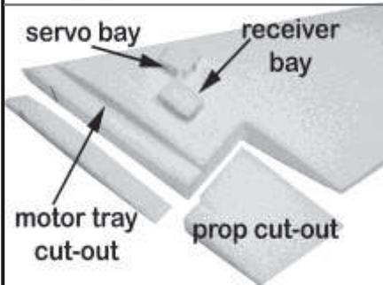
There are four important pre-cut features on the wing panels. The motor tray cut-out, the servo bays and the receiver bays. There are two receiver bays. One on each side. The bottom side of the wing has a pre-cut spar channel. The spar channel extends in a straight line across both wing panels.
