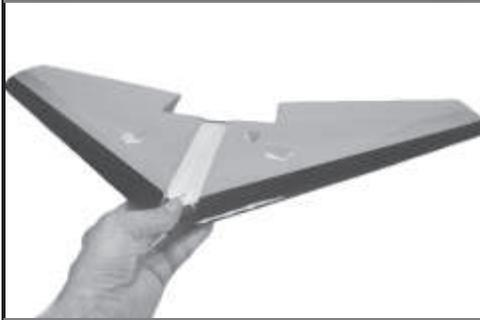
Place the wing in the top beds bottom-side-up. Cover and trim the bottom of the wing one panel at a time. Apply color tape working from the TE to the LE. The final strip of tape is wrapped around the LE from top to the bottom. Cut an "X" pattern in the tape covering the servo and receiver bays. Fold the tape into the servo and receiver bays. Fit the servos in place. Cut away any tape that prevents entry.
