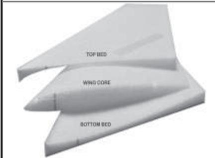
There are three parts to each wing panel. The top of the wing can be identified by its greater curvature. The left wing is the wing that would be on your left if you were in the cockpit. The right and left panels can be identified by the color mark at the root (the big end of the wing panel): Red on the right.
