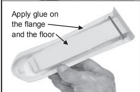
Brush on some glue to the outside of the motor tray floor. Apply glue to the underside of the flange of the motor tray that makes contact with the top of the wing.
