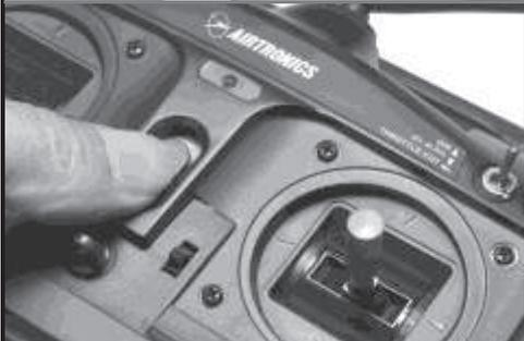
Power-up the TX. Check the TX battery condition. Charge or replace batteries if necessary. Always power-up the TX before powering-up the RX.
