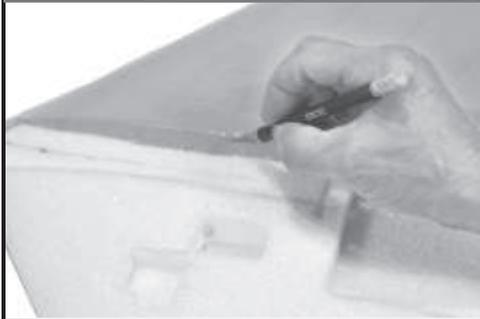
Fold the tape around the motor tray cut-out so that it sticks to the inside wall of the cutout. Clear the servo wire hole drilled earlier. Trim and remove tape from the cut-out floor. Repeat the covering process on the top side of the other panel.
