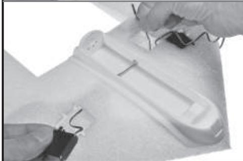
Do not glue the motor tray in at this time. One of the servo wires must cross inside the motor tray. The RX, servos and servo wire must remain removable for service. Cut holes in the side of the motor tray to correspond to the servo wire holes drilled in the wing panels. Use a wire to fish the servo wire through to the RX bay. 2.4G, two module receivers require a connection wire between both RX bays.
