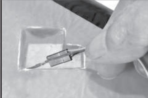
Twist or tape the servo plug to the fish-tape. Pull the right side servo wire through the motor tray into the RX bay.
