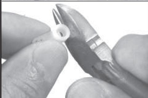
The Hitec HS-81 analog micro servo is moderately priced with adequate torque. The servo bay may be expanded or shimmed to fit a different size servo. Find the X-shaped control arm with four tabs in the parts bag supplied with the servo. Remove three of the tabs leaving only one.
