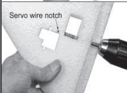
Remove the servo bay and the receiver bay cookies from the wing cores. Remove the motor tray cutout. Use a 1/4" drill. Drill into the vertical surface of the motor tray cut-out through to the servo bay. The hole should end at the servo wire notch in the servo bay.
