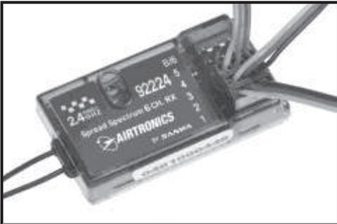
2.4G radio systems must bind to the transmitter. Most 2.4G receivers have a specified slot for binding. The ESC should be plugged into the throttle slot in the RX after binding is done. 72 MHz do not need binding. Refer to your radio instructions for radio binding procedures and RX slot assignments. Refer to your radio instructions for the mixing functions. Look for “delta mix” or “elevator mix”.
