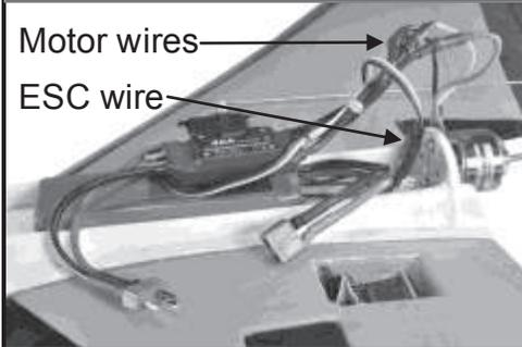
Install the battery all the way forward in the battery bay and press it in place. Press the ESC in place on the top of the battery. Plug the three ESC bullet connectors together with the three motor connectors. Plug the ESC ribbon connector into the RX throttle extension wire. **DO NOT INSTALL THE PROP!**
