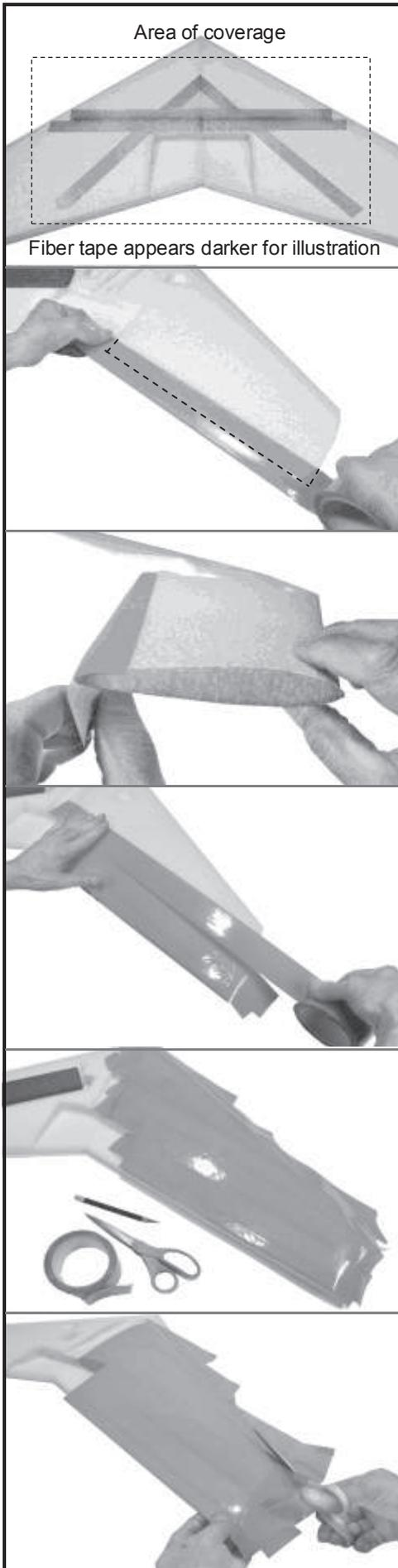
Spray a light coat of adhesive on the bottom side of the wing. Let the adhesive dry for 15 minutes to allow the solvent and propellant to evaporate before taping. Apply four strips of fiber filament tape to the wing following the pattern pictured left. TIP: *The way to determine that the glue is dry enough to apply the tape is when the glue will not come off on your finger with a light touch.*
