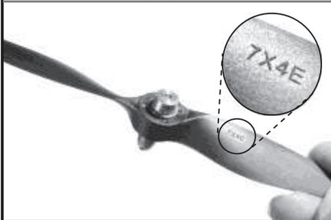
Install the prop for balancing. Assemble the prop with the appropriate insert. The “7X4E” lettering on the prop blades should be facing toward the motor.
