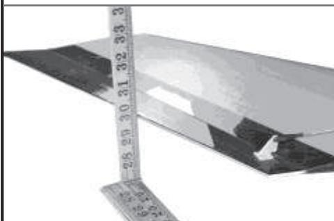
Adjust the throw settings of the elevons. Remove the prop. Turn the transmitter on and then the receiver. Set the wing on a couple of rolls of tape. Hold a ruler near the elevon. Pull the elevator stick back to the full up position. The travel should be 1/4”. The full down travel should be the same. Push the stick to the full right position. The elevon travel should be 1/4” and down 1/4”.
