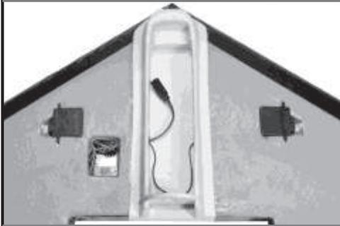
Press the servos into the servo bays. Insert the antenna wire into the antenna tube. Press the RX into the RX bay. Plug the servos and ESC extension into the RX. Roll-up the extra wire from the left servo and stow it in the cutout.
