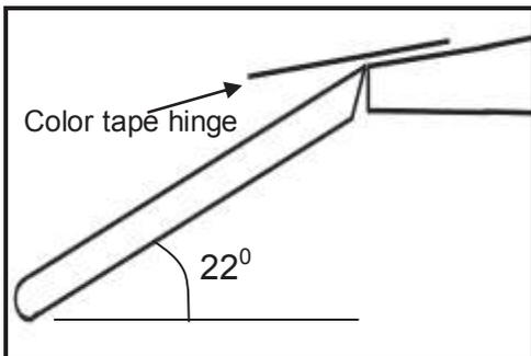
Position the wing with the TE on the edge of the work-bench. Use a strip of color tape to make the top elevon hinge. Apply the tape to the top of the wing so that half of the width extends beyond the TE. Align the elevon with the placement reference marks. Hold the elevon at about a 22 degree down angle and slide the elevon along the TE up to the hinge tape. Press the hinge tape to the elevon.
