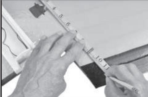
Position a straightedge from the outboard side of the servo control arm to the elevon. The line should be parallel to the center line. Make a mark on the elevon. That is where to center the control horn.
