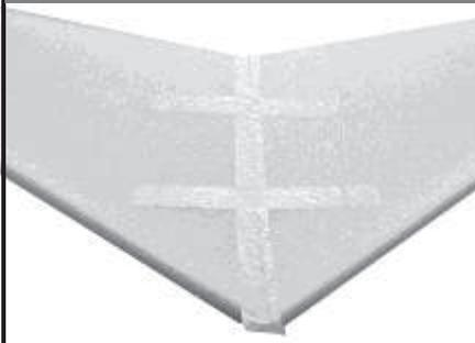
Use fiber tape to tape the two bottom beds together. Then tape the two top beds together. Remove the hairs and zigzags from the wing cores and beds by rubbing them with a scrap piece of EPP foam. Lay the bottom right and left wing beds on a flat surface. Set the wing cores on the beds and lightly block sand the wing panels (cores) with #100 or #80 sandpaper.
