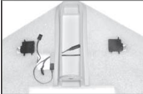
Locate the servo extension wire in the parts bag. The extension wire is for the ESC hook-up to the RX.
