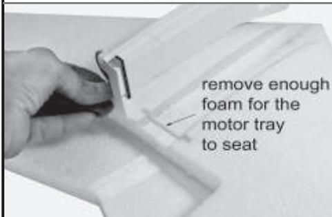
Fit the motor tray to the motor tray slot. Align the rear tab of the motor tray with the rear of the motor tray cut-out. Notice that the motor tray will not seat because of the plywood motor mount. Press the rear of the motor tray hard enough to make an impression on the foam beneath. Lift the tray and remove two small notches from the wing and a shallow slot across the bottom of the motor tray cut-out to seat the plywood motor mount.
