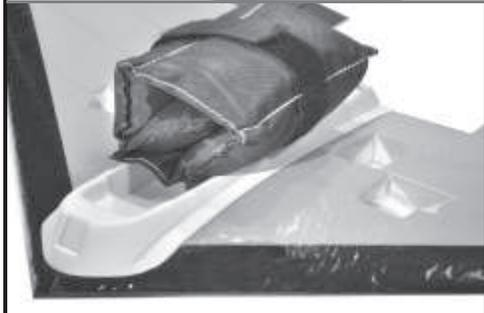
Let the glue dry for about 15 minutes. Push the motor tray in place. Put a weight in the motor tray to make sure it bonds to the foam underneath. Pictured here is a 5 pound exercise weight.
