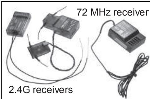
2.4G radios have shorter antenna wire and often use an array of two antenna wires. Some 2.4G receivers have two separate RX modules connected by a wire. 2.4G radios do not have channel numbers and must bind to the TX. 72 MHz radios has one long antenna wire. The 72 MHz RX uses a crystal to tune the TX to the RX and has a channel number.
