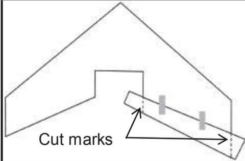
Use two small pieces of masking tape to temporarily hold the elevator in position against the TE. Hold a straight-edge against the wing tip. Make a mark on the elevator to continue the line of the wing tip. Make a second mark inboard to continue the line of the prop cut-out. Repeat this procedure for the other side. Trim and sand the ends of both of the elevators at the pencil mark.
