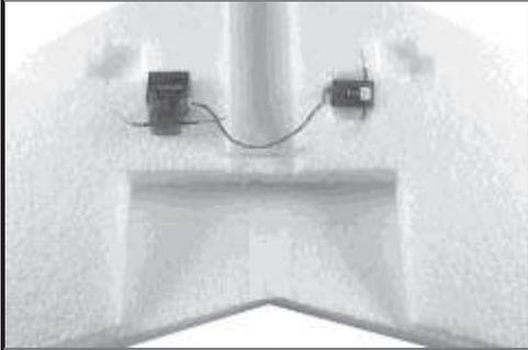
The Zagi 33 has two receiver bays to accommodate a two module receiver system provided by some 2.4G radio manufacturers. Notice that the antenna array is positioned 90 degrees to each other as specified.
