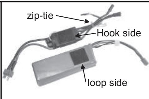
Measure 1/2" from the end of the battery and make a mark. Apply a loop side Velcro square to the battery on the mark. Peel and stick the hook side of the Velcro on the center of the ESC on the side opposite the label. Roll up the RX wire and bundle the excess wire together with the motor hook-up wires. Tape or zip-tie the wires all together.
