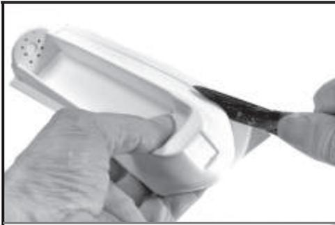
Cut the motor tray along the cut-line around the front and both sides. Do not remove the tab that extends down at the rear of the motor tray. Use sandpaper to dress the underside of the flange that makes contact with the wing to remove any part of the cut-line that remains.
