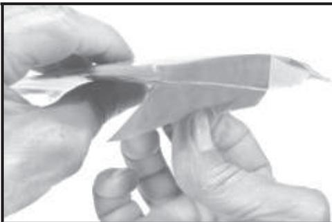
Fold the tape around the tip and cut it to the contour of the bottom surface. Spray a light coat of 77 Adhesive on the bottom surface of the wing.
