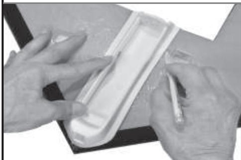
Fit the motor tray in the motor tray cutout. Make a pencil outline around the perimeter of the motor tray. Use enough pressure to make an impression with the pencil.
