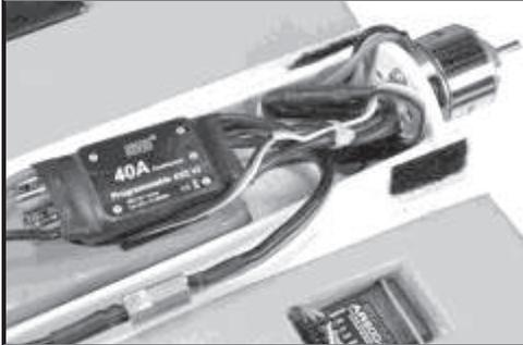
Rollup the motor and ESC wires tight enough to stow between the battery and the motor mount.
