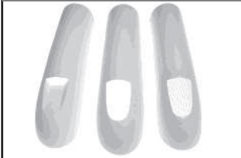
The vent hole in the canopy helps extend the performance and life of the battery and ESC by providing cooling air flow. The vent may be cut in different configurations. (left), Remove the rear bulkhead of the vent. (center), Remove the entire vent. (right), Remove the entire vent and hot-glove a piece of metal window screen inside the canopy.
