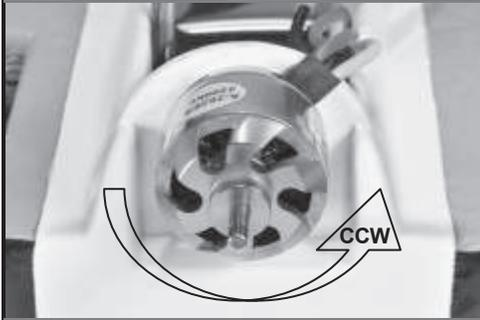
Test the motor without the prop. Check the TX and RX batteries. Power-up the TX. Set the TX throttle stick the full low motor (down) position. Plug the ESC's two terminal Deans male connector into the battery. Move the throttle stick forward until the motor moves. The motor should turn counter-clockwise; (CCW) when viewed from the rear. Reverse any two of the three motor wires to reverse the direction.
