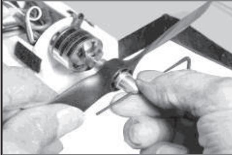
A 1/16” allen wrench may be used as a tightening tool for the prop hub. Put the allen wrench through the hole in the hub. Hold the hub and wrench between your fingers and turn the hub tight. Do not turn hard enough to bend the allen wrench.
