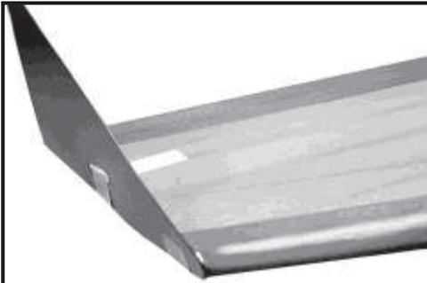
Put a piece of fiber filament tape through the winglet slot to the top of the wing and wrap it around to the bottom of the wing. Add two more pieces of tape to secure the winglet in place. Make sure that the elevon will not bind against the winglet as it moves.
