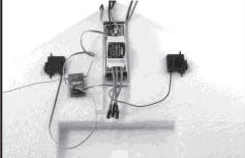
The servos must be centered before installation. Lay out the receiver (RX), battery, servos and ESC in roughly the configuration that they will be in the wing. Layout the components on the wing as shown. Make sure to position the servos with the lead wire and the control arm toward the back. **DO NOT HOOK-UP THE MOTOR TO THE ESC!**
