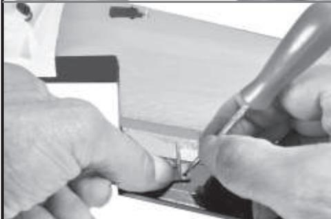
Center the control horn on the line on the elevon. Use a punch or any pointed tool to mark the position of the holes in the control horn foot. Drill two holes big enough for the 2 x 56 self tapping machine screws. Thread the machine screws through the elevon into the nylon locking pad. Snug the screws down enough to make a slight impression in the balsa wood. Do not over tighten!
