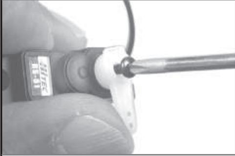
Remove the round servo control arm. Avoid stressing the gears by holding the edges of the round control arm to prevent travel when removing and replacing the screw. Do not over tighten the screw. Snug is tight enough. To maximize servo life, never move the servo control arm with the radio off.
