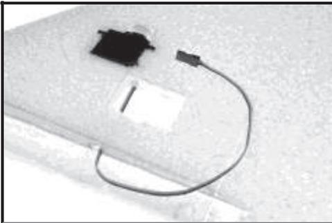
The hole should be large enough for the servo plug to fit through. Cut a notch in the receiver bay cookie large enough for the servo wire to fit through. A servo can be used to test the size and fit. The servo bay size may be adjusted for a servo that is larger or smaller than the die-cut. Add shims for smaller servos or cut away some foam for larger servos. Remove the servo and replace the cookies.
