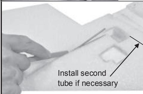
Make a 1/2" deep slot 6" on the mark. Push the tube into the slot with a popsicle stick or a 1/16" scrap of wood. Glue is not necessary. An additional tube may be installed for an RX that has two antenna that are the same length. Install the second tube perpendicular to each other as recommended in the radio manual.
