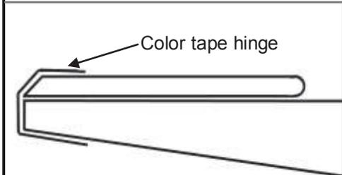
Rotate the elevon to the top of the wing and temporarily tape it to the top of wing with a piece of masking tape. Apply another strip of color tape to the bottom of the elevon. Make sure that it wraps around the elevon and the wing TE.
