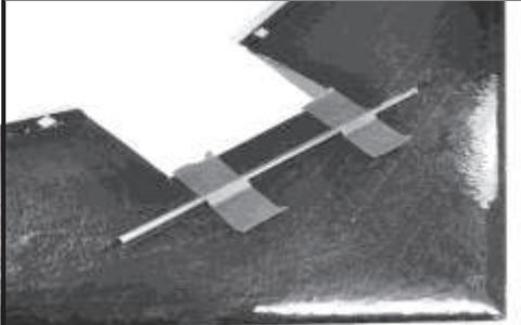
Lay the wing bottom-side-up. Tape a 1/4” dowel 7-3/8” inches back from the nose, That’s 3/8” forward of the carbon spar. A round pencil can be used as a balance tool.
