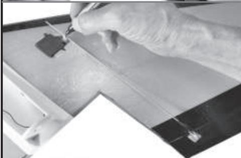
NOTE: Make sure that the servos are centered with the radio on and with the trim levers centered.
