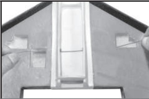
Thread a fish-tape made of flexible thin wire from the receiver bay to opposite servo bay. Pass the fish-tape through the motor tray holes drilled earlier. Pictured here is a 9 inch length of plastic coated twist-tie wire.
