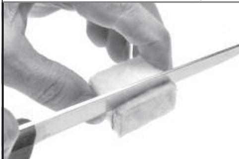
Remove the cookie from the RX bay. Make a mark 1/4" from the bottom on all four sides. Cut the 1/4" piece off. Dab the edges of the 1/4" slice and fit it in the RX bay from the bottom. When the RX bay floor is in place, the bay can be expanded to fit a larger RX.
