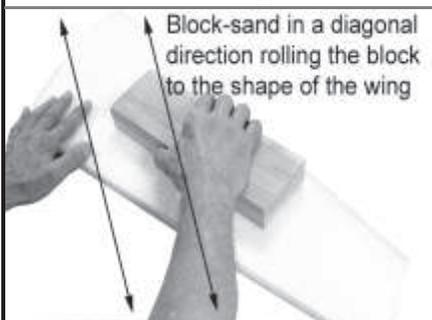
Block-sand the panels in a diagonal direction to avoid making flat spots. Roll the block to follow the contour of the wing surface. Take about 50% of the shine off of the foam. Put the wing panels in the top beds and sand the bottom of the wing. Be very careful when sanding the leading edge (LE). Do not flatten or sharpen the leading edge. Block-sand gently while rolling the block around the leading edge.
