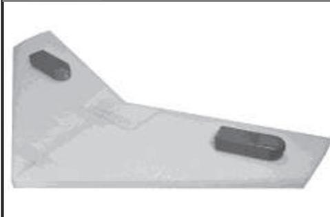
Place the top beds on a flat surface. Put the wing cores in the beds bottom-side-up. Press the panels together so that the spar channels on both panels are aligned. Fiber tape can be used to hold the wing panels together. Use weights to hold the wing in alignment.
