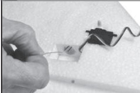
Straighten a paper clip leaving one small bend at the end. Heat the end of the clip with a torch lighter or stove. Use the heated end of the wire to hollow out a cavity to stow the extra lengths of servo wires. Work slowly with repeated heating of the wire. The cavity might need enlarging at final assembly.
