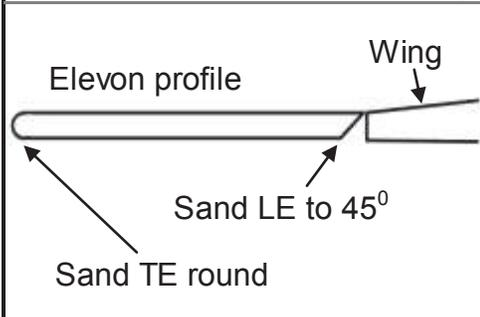
Sand a 45 degree angle into the LE of the elevator (the LE is the edge of the elevator that makes contact with the wing). Sand the elevators and smooth all the surfaces. Round the TE and both ends of the elevators. Spray the elevators with adhesive and cover them with color tape.
